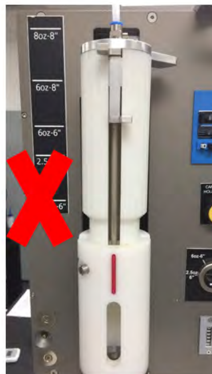
Cap Assembly in WRONG position
